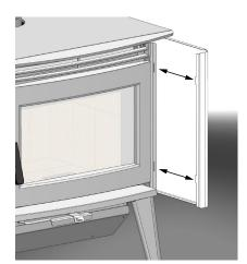
Figure 4. AB25.Side panel tab install.
