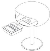
Using the lifting handles, place the filled combustion chamber inside the mout plate opening. The fireplace is now ready for use.
