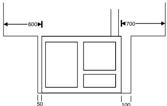
Conclusion: 50 100 When installed as described above, the appliance tested complied with the requirements of AS 2918:1990.
