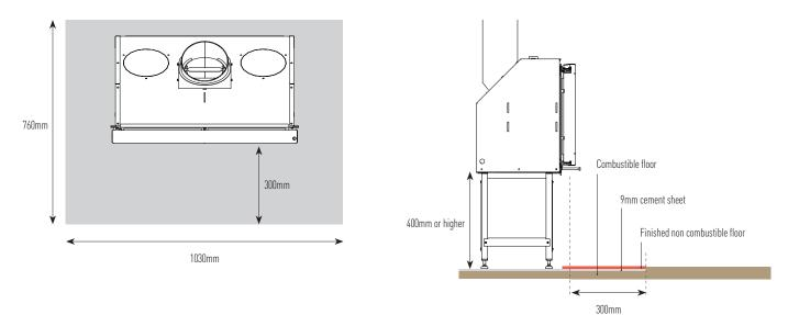
Floor protector must be minimum 9mm thick cement sheet (excluding non combustible floor finish)
