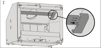
The default position of the vermiculite deflector housing is the highest position. If you have a "lazy'" chimney, you can lower the housing to the second or third notches (figure 2).
