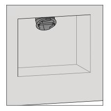
Install the flexible or solid flue so that is comes out close to where the appliance outlet will be located. Attach the smoke outlet connection provided with the fireplace (if using a flexi flue, use a metal duct clamp - not provided).
