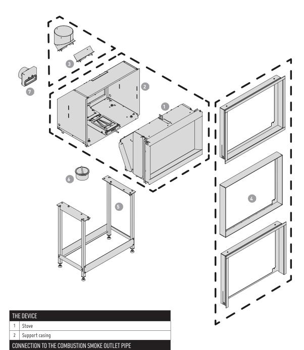
3 Smoke outlet connection piece (vertical or 45° angle)
