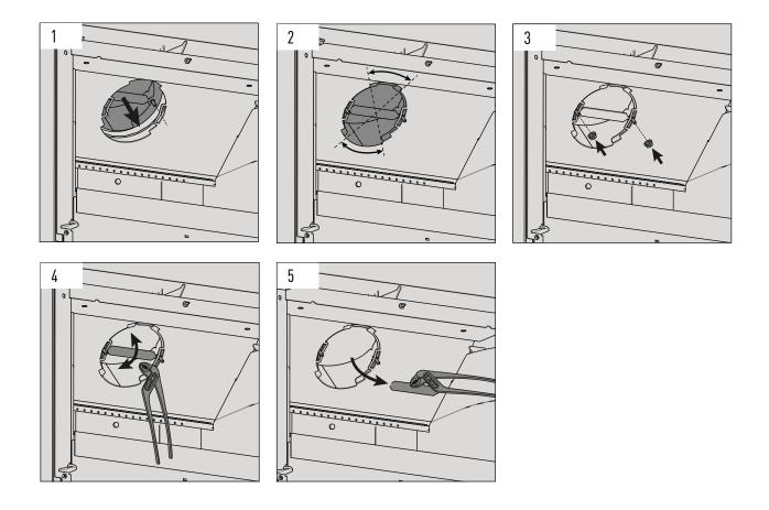
Hold the smoke outlet connector (which has already been connected to the duct) by the handle and attach it to the stove [figures 1 & 3]
