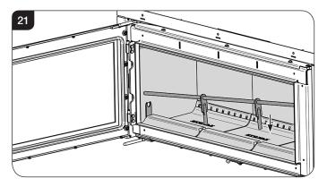
Slide the Log Guard across so both ends locate evenly in the holes in the side bricks, see Diagram 22.
