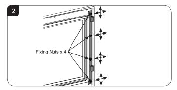
4a.5 Loosening the Door Hinge Assembly allows for fine vertical and horizontal adjustment of the door position. This may require a trial and error approach to find the correct position. Ensure the door is horizontal before tightening the fixing
