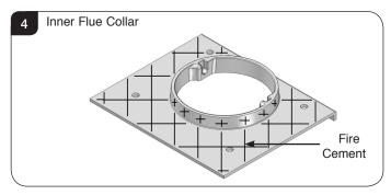
4.3 Fit the inner flue collar using the 4 x bolts ensuring the top hat spacers are replaced on the 2 x longer front bolts, see Diagram 5 and all bolts are finger tight only.
