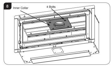
5.3 First remove the inner collar. Using a 13 A/F spanner, remove the 4 x bolts, see Diagram 9.
