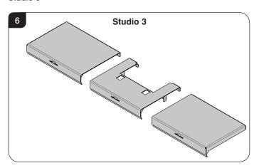
The Studio 3 baffle comes in three sections. To remove the baffle system the baffles must be taken out in the following order:
