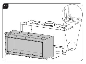
Pull the inner box carefully forward to release from the cutouts. It should now slide smoothly out of the outer box
