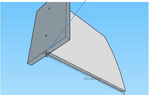
Join the template together with nails or screws from the rear in 2 places
