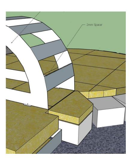
To start building your door arch only butter the bricks to 2-3 mm between bricks and Tap down gently.
