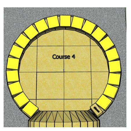
By now it's a good time to infill the rear of the chamber bricks with fondu – mix your batch and infill the rear of the chamber to strengthen it.
