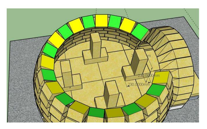
Using 8 common house bricks  $230 \times 115 \times 75$ mm create 4 positions evenly spaced for the top templates to rest upon.
