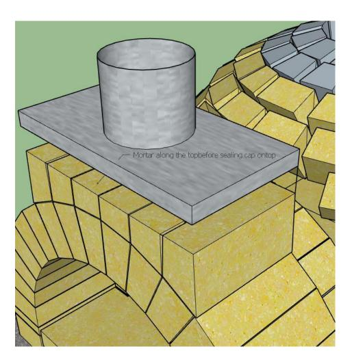
Use the airset mortar to hold the flue in place
