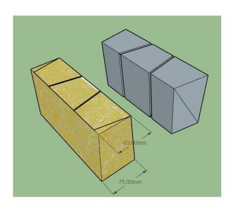
With the 1 x 633 brick provided mark the 63 side of your brick with the equivalent side of your 633 brick the cut ... You will end up with 3 x 633 bricks per 230 x 115 x 75/63 full brick
