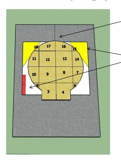
Starting from the rear edge of the calcium silicate board and in the middle join lay your tiles in the following pattern loosely
