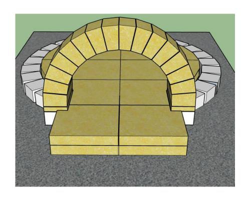
When you have finished the door arch leave the template in for at least an hour before removing it. You can also leave it in while building the chamber if you like.
