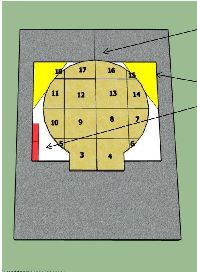
Starting from the rear edge of the calcium silicate board and in the middle joint lay your tiles in the following pattern loosely
