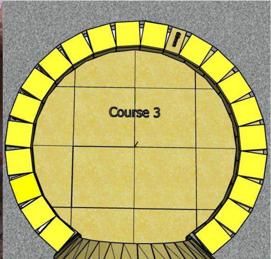
Using the chamber template as a guide from the centre of the oven rotate it around and lay your bricks in the pattern for the second layer Make sure you lean the bricks against the template guide to correctly set the angle
