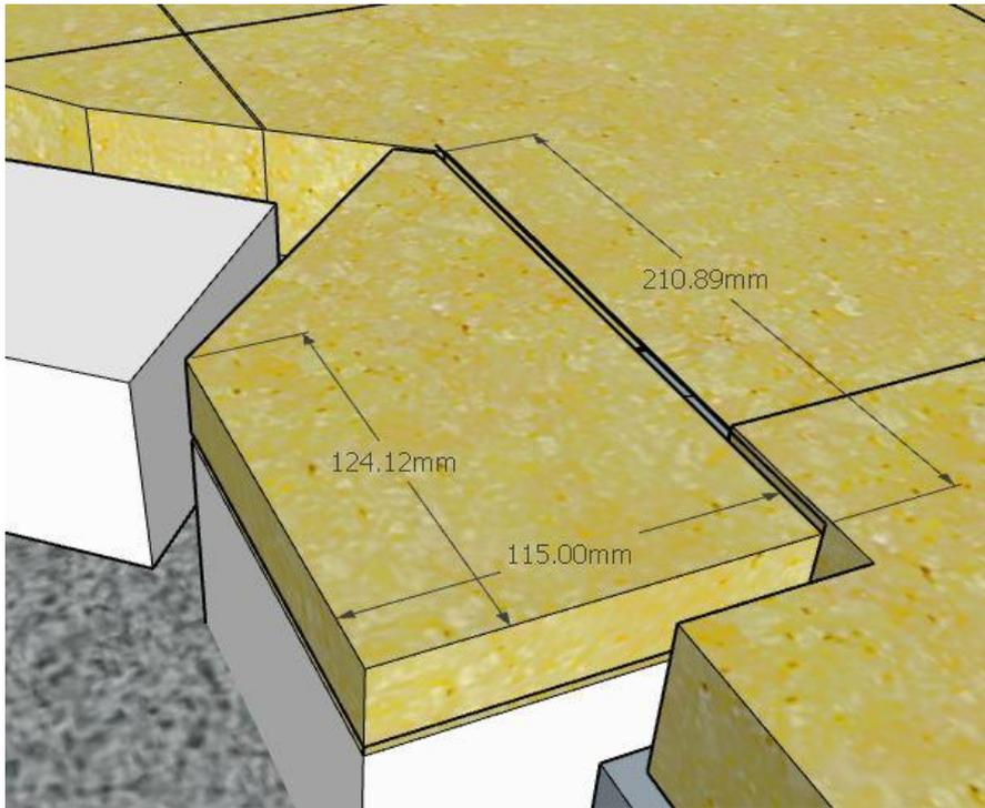
Your door arch bricks are to be cut with a taper in the back to create a join in which the chamber bricks meet perfectly
