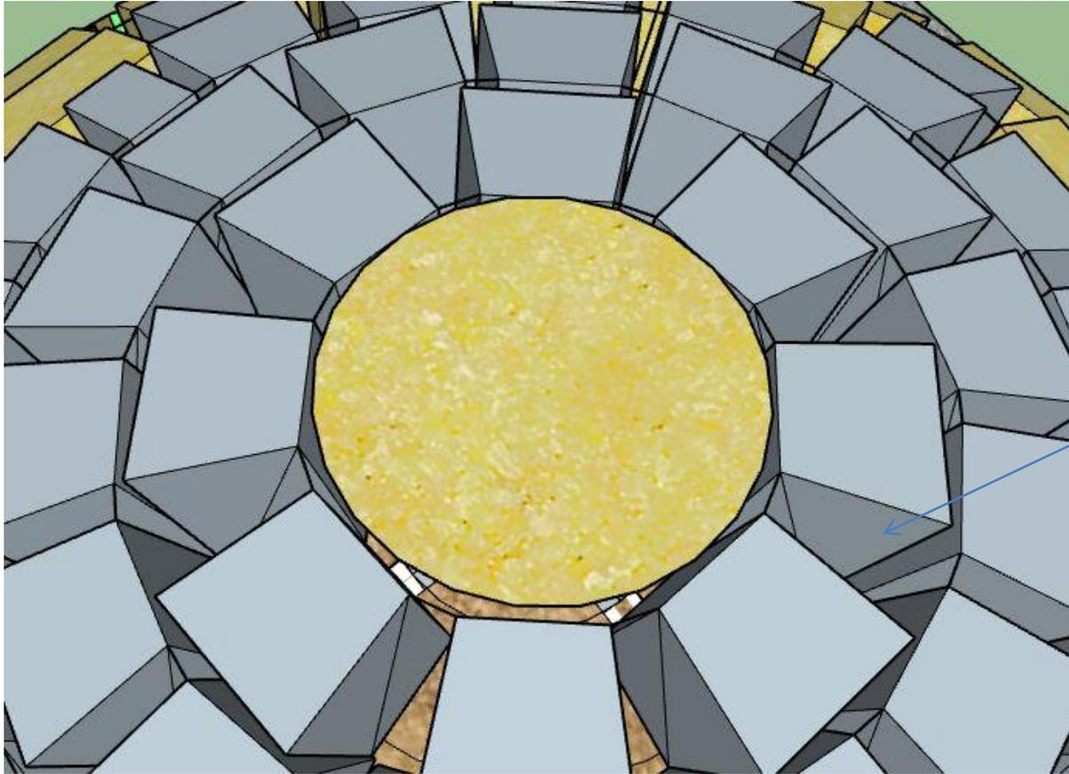
For the keystone mix some CAST 13 in a bucket and pour into the top to lock the entire structure together.
