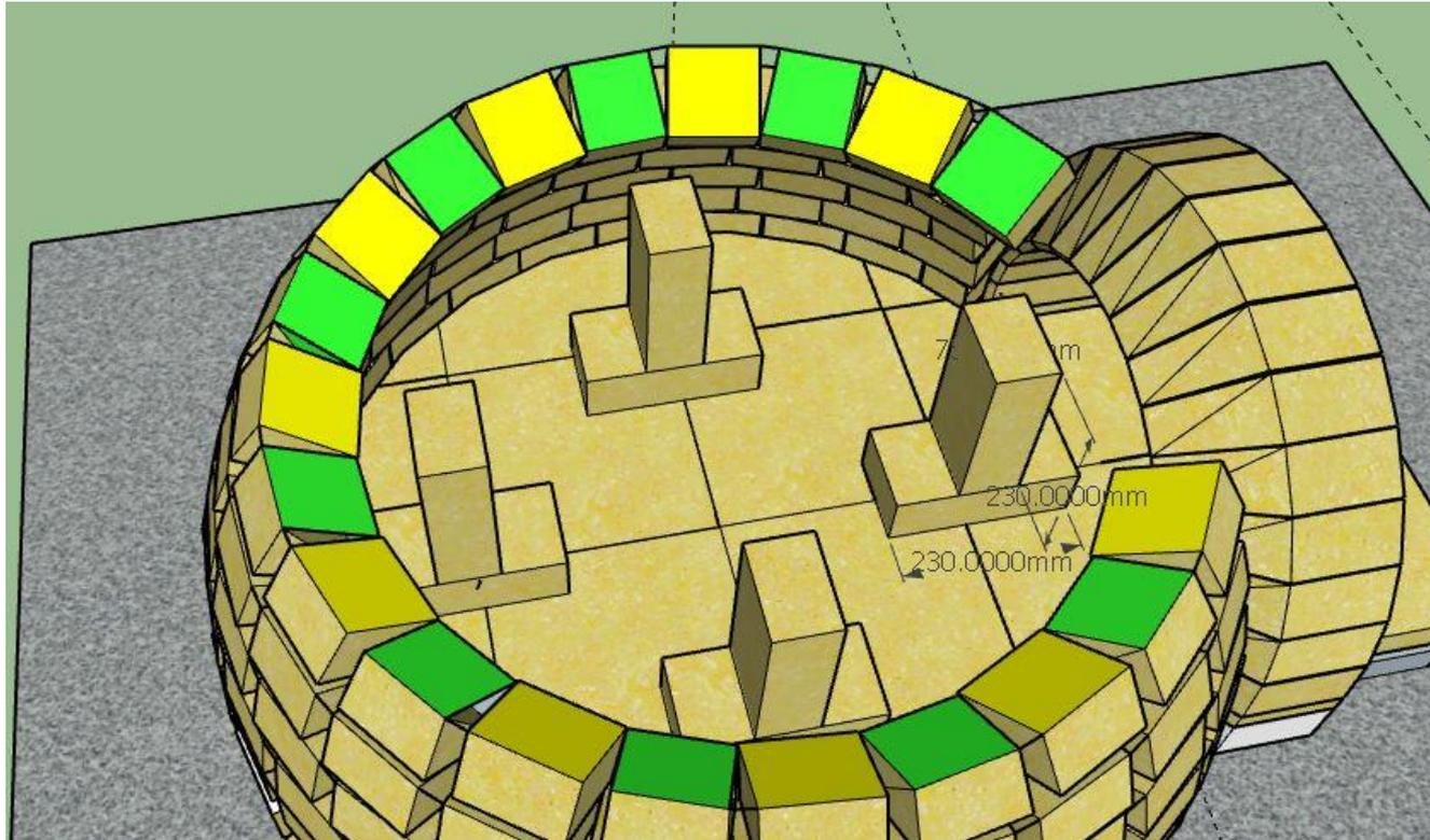
Using 8 common house bricks 230 x 115 x 75mm create 4 positions evenly spaced for the top templates to rest upon.
