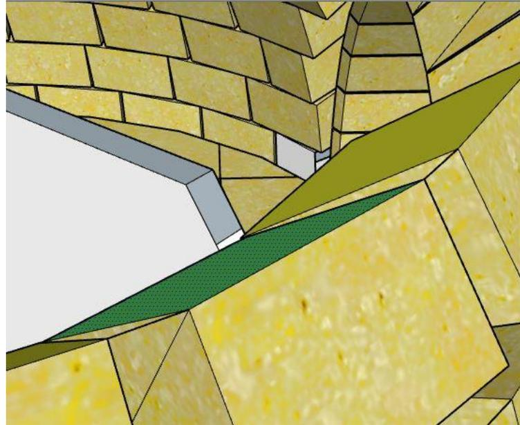
The 6<sup>th</sup> layer is your final layer before the plug to build the top of the oven.
