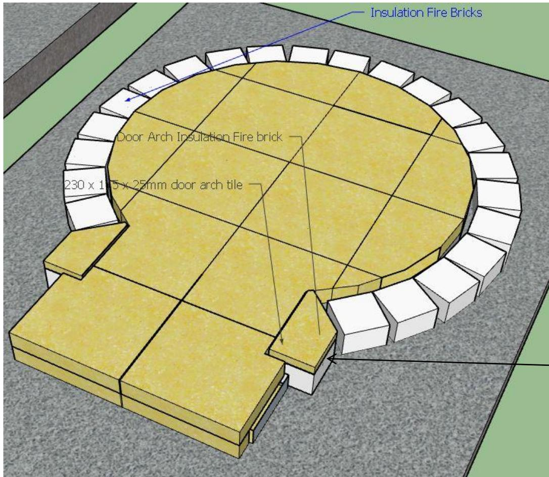
Your first layer of firebrick on the floor for your chamber consists of a White IFB. This is a strong brick that prevents any heat transfer to the slab. It also is waterproof and will never fail over time in any condition. Calcium silicate boards as a structural layer collapse over time.
