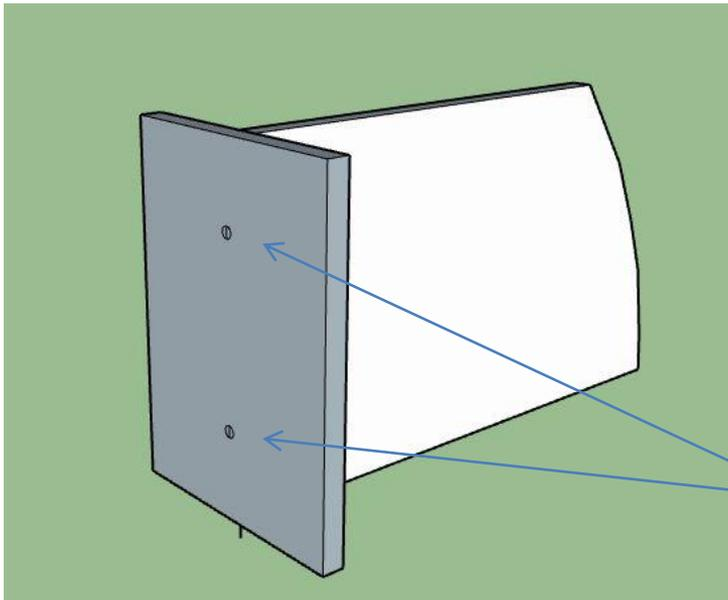
Join the template together with nails or screws from the rear in 2 places
