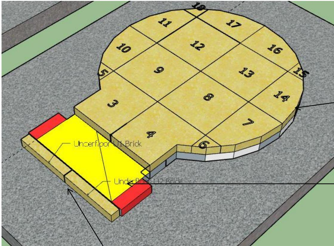
With a handsaw trim around the perimeter of the floor tiles cutting the calcium silicate board flush to the tiles ..
