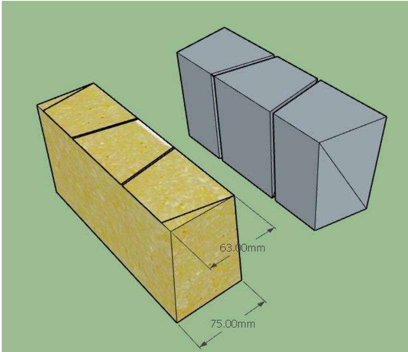
With the 1 x 633 brick provided mark the 63 side of your brick with the equivalent side of your 633 brick the cut ... You will end up with 3 x 633 bricks per 230 x 115 x 75/63 full brick
