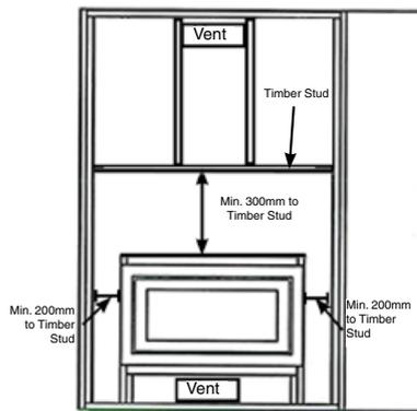
**MUST USE NON-COMBUSTIBLE MATERIALS 315MM ABOVE THE UNITS OUTER SHELL (REDUCED CLEARANCE BOX), 200MM FROM THE SIDES OF THE OUTER SHELL AND ALL BELOW THE HEATER.**
