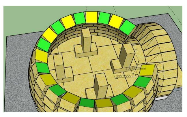
Using 8 common house bricks 230 x 115 x 75mm create 4 positions evenly spaced for the top templates to rest upon.
