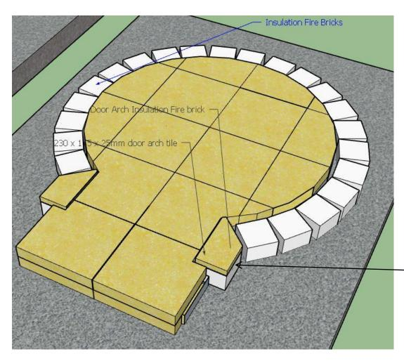
Your first layer of firebrick on the floor for your chamber consists of a White IFB. This is a strong brick that prevents any heat transfer to the slab. It also is waterproof and will never fail over time in any condition. Calcium silicate boards as a structural layer collapse over time.
