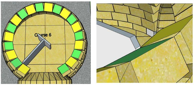
The 6<sup>th</sup> layer is your final layer before the plug to build the top of the oven. Check layer 6 meet the top of the 2<sup>nd</sup> last notch in the template
