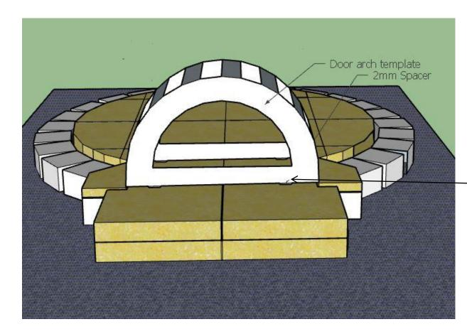
Screw or nail your door arch template ( smaller ) together using timber at approximately 180mm long - only 6 battens needed.
