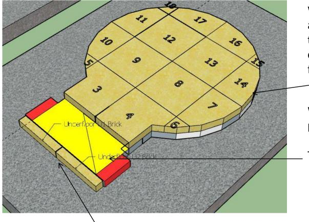
With a handsaw trim around the perimeter of the floor tiles cutting the calcium silicate board flush to the tiles ..
