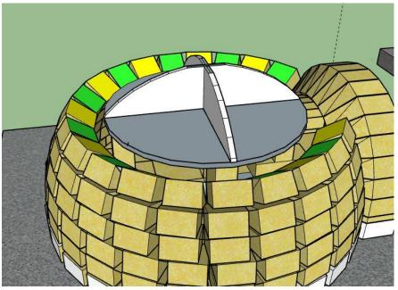
The top chamber templates simply interlock and are to be placed upon the 8 bricks with the centre line running from front to back.
