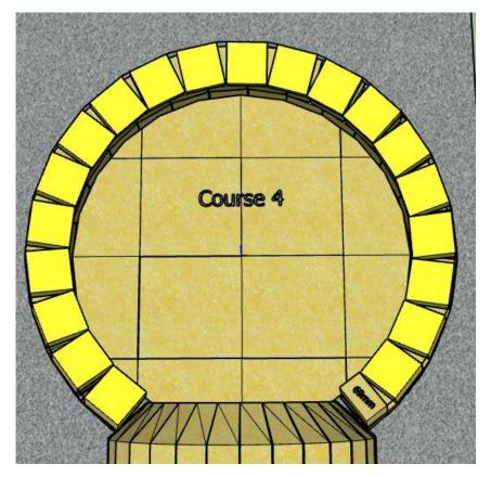
By now it's a good time to infill the rear of the chamber bricks with fondu – mix your batch and infill the rear of the chamber to strengthen it.
