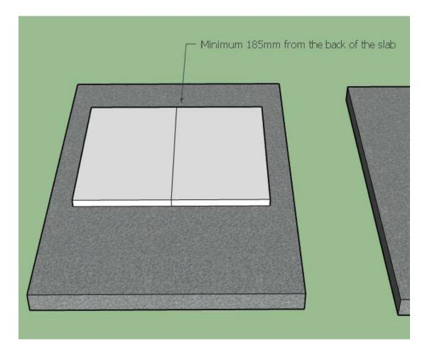
Lay your calcium silicate board in the center of the slab and 185mm from the rear of the slab
