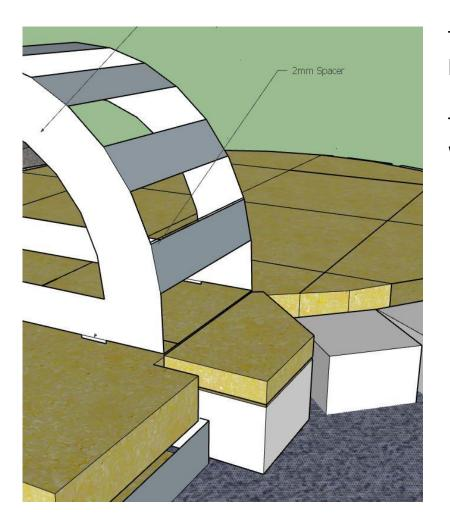
To start building your door arch only butter the bricks to 2-3 mm between bricks and Tap down gently. This will bring your door arch support bricks level With the bottom of the door arch template
