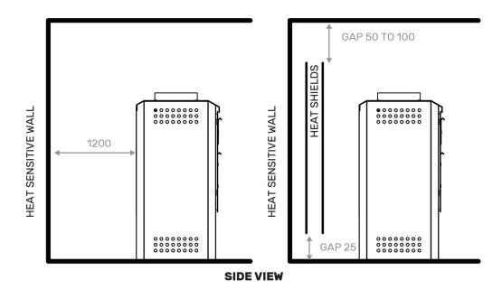
Wall shields must be made from heat-tolerant material (allowable service temperature greater than 150°C but less than 600°C).
