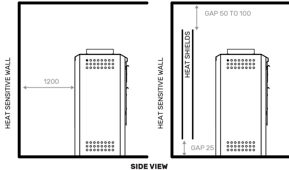
Wall shields must be made from heat-tolerant material (allowable service temperature greater than 150°C but less than 600°C).
