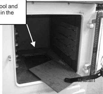
With the scrapping tool pull any soot or tar granules into the open space.
